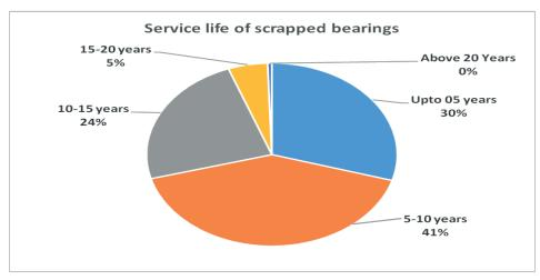
Above age analysis shows that 4,481 bearings (71 per cent) were scrapped as defective within half of their codal<sup>222</sup> life. Out of that, 1,872 bearings had failed before completion of five years (i.e. onefourth of codal life) from date of manufacturing. This raises doubt about the quality of the bearings supplied to the Railway.
